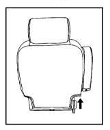
Lift the lever, located on the bottom rear of the second row seat on the inboard side, to release the seatback. The seatback will fold forward.
