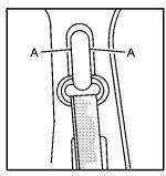
Squeeze the buttons (A) on the sides of the height adjuster and move the height adjuster to the desired position.
