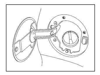
The tethered fuel cap is located behind a hinged fuel door on the driver side of the vehicle. If the vehicle has E85 fuel capability, the fuel cap will be yellow and state that E85 or gasoline can be used. See *Fuel E85* (85% Ethanol) on page 6-9.
