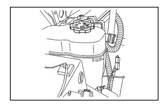
The coolant surge tank is located in the engine compartment on the passenger side of the vehicle. See *Engine Compartment Overview on page 6-16* for more information on location.
