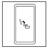
2. Press the automatic seat release button located on the panel behind the rear doors.
