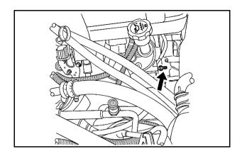
The remote negative (-) terminal is a stud located on the right front of the engine, where the negative battery cable attaches.
