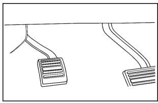
Set the parking brake by holding the regular brake pedal down, then pushing down the parking brake pedal.
