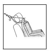
If the position you are using has an adjustable headrest or head restraint and you are using a dual tether, route the tether around the headrest or head restraint.
