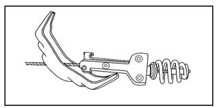
Tilt the tire toward the vehicle. Separate the tire/wheel retainer (G) from the guide pin. Pull the pin through the center of the wheel. Tilt the retainer down through the center wheel opening.
