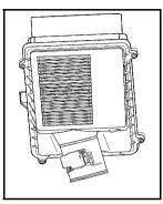
Locate the air cleaner/ filter assembly . See Engine Compartment Overview on page 6-16.
