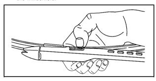
Squeeze the grooved areas on each side of the blade, and turn the blade assembly away from the arm connector.
