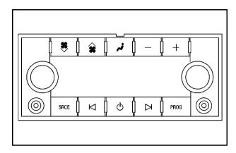
(Power): Press the U button to turn the RSA on or off.
