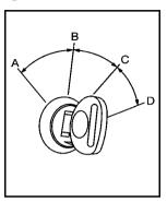
The ignition switch has four different positions.
