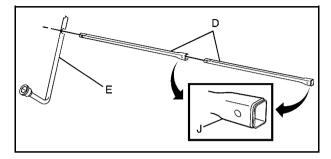
3. Assemble the two jack handle extensions (D) and wheel wrench (E) as shown.
