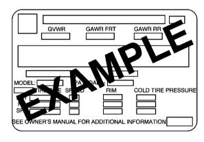
A vehicle specific Certification/Tire label is found on the rear edge of the driver's door. The label shows the size of your vehicle's original tires and the inflation pressures needed to obtain the gross weight capacity of your vehicle.
