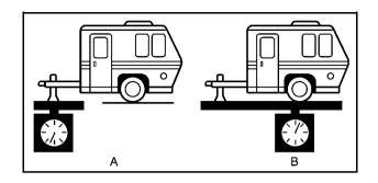
Trailer tongue weight (A) should be 10 percent to 15 percent and fifth wheel or gooseneck kingpin weight should be 15 to 25 percent of the loaded trailer weight up to the maximums for vehicle series and hitch type shown below:
