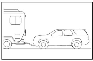
Use the following procedure to dinghy tow a four-wheel drive vehicle with a two speed automatic transfer case:
