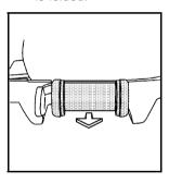
Unlatch the seat from the floor by pulling the carrying handle, located at the rear of the seat, rearward.
