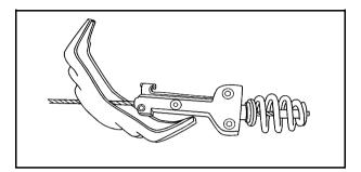
Once the retainer is separated from the guide pin, tilt the retainer and pull it through the center of the wheel along with the cable and latch.
