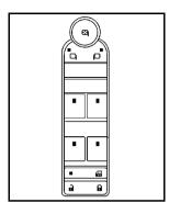
The power window switches are located on the driver door.
