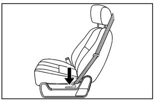
If equipped, this control is located on the outboard side of the seat.
