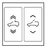
There are two switches in the overhead console that operate the sunroof. Manual-Open/Manual-Close: To open the sunroof press and hold the rear of the driver's side switch until the sunroof reaches the desired position. To close the sunroof, press and hold the front of the driver's side switch until the sunroof reaches the desired position. The sunshade will open automatically with the sunroof, but can also be opened manually.
