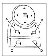
Vehicles with outside power foldaway mirrors have the controls located on the driver door armrest.
